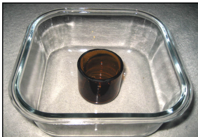
Test #1 using a small reactor. The liquid surface area is much too small in comparison to the large liquid surface area of the receiver container.
