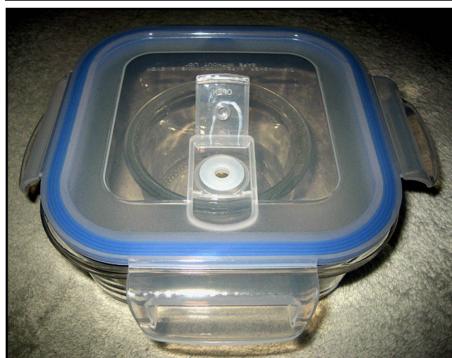
Test #1 using a small reactor. The liquid surface area is much too small in comparison to the large liquid surface area of the receiver container.
