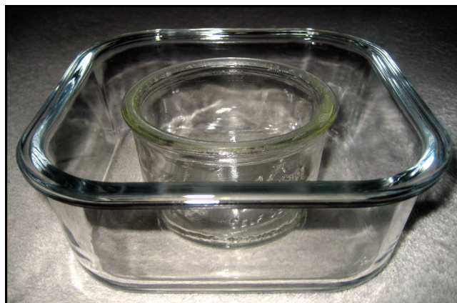
750 ml capacity glass storage container used as CDS receiver. Cut-down 8 fl oz glass canning jar used as CLO2 reactor. Receiver gross liquid surface area=15,000 sq mm. Net area=9720 Reactor liquid surface area=3400 sq mm.
