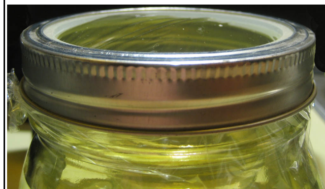
Plastic LDPE 'lid' dome shape caused by expanding CLO2 gas when making CDS.
