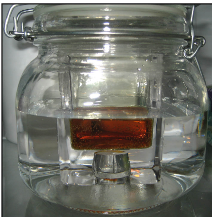
CDS +2 minutes in fridge. All solutions and containers were at room temperature. 360 ml filtered water + 18 ml 4% muriatic acid (new) + 18 ml MMS. 23feb'20 @1235 Receiver is 750 ml capacity. MMSinfo.org
